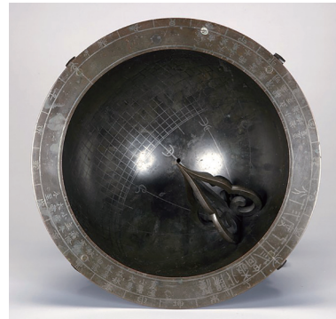
Fig. 9. <양부일구仰釜日晷> Hemispherical sundial, After the 18 th century, Chosŏn, Brass, W. 24.3cm, H. 10.0cm, National Palace Museum ( http://gogung.go.kr )
